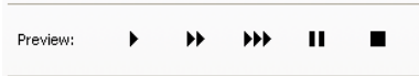
Figure 18 Buttons for play back of a sequence, play (speed x1, x10, x100), pause, stop
