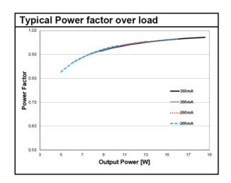
ELEMENT 18220-240350 D CS L Typical Power Factor vs. Load
