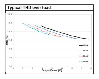
ELEMENT 18220-240350 D CS L Typical THD Vs Load
